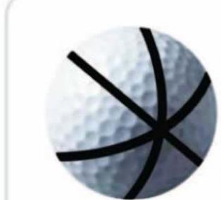
Specially patterned balls were developed in order to measure spin.
